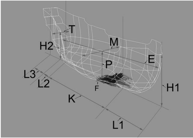
**Fig. 1.** Basic diagnostic dimensions of a ship: K – Keel length, L1 – Spring of the stem post, L2 – Rake of the sternpost, L3 – Span of the counters and stern castle bulworks, H1 – Height of the stem post, H2 – Height of the sternpost, T – Width of the transom, M – Maximum beam (in Spanish *Manga*), F – Flat amidships (in Spanish *Plan*), P – Depth of hold (in Spanish *Puntal*), and E – Length on the upper deck (in Spanish *Eslora*) (Kevin Gnadinger and Filipe Castro).
