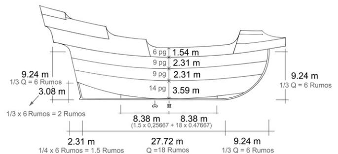
**Fig. 4.** A profile of the Pepper Wreck with some of the measurements indicated in Oliveira's treatise and the presumed positions of the ship's decks. The measurements indicated do not include the thickness of the pavements, which was slightly over 1 *palmo de goa* per deck (Filipe Castro).
